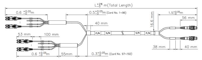
MPO: Telcordia GR-1435-CORE Issue2, IEC 61754-7 and TIA-604-5 interface compliant ULC: Telcordia GR-326 Issue4, TIA/EIA-604-10 (FOCIS-10) and IEC 61754-20 compliant All: RoHS compliant, All plastic connector materials are UL94 V-0 flammability rated
