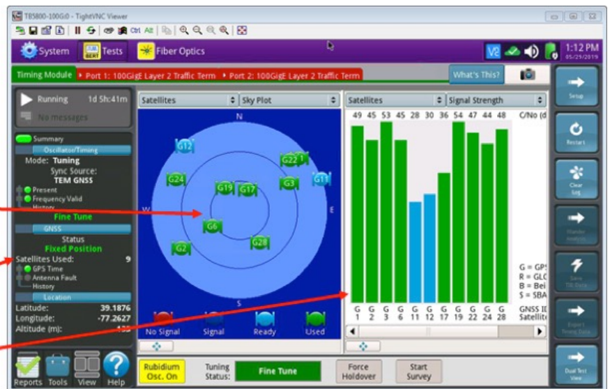
Figure 14 - GPS Test using VIAVI T-BERD/MTS-5800
